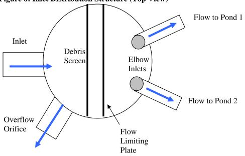
**Figure 6: Inlet Distribution Structure (Top View)**
